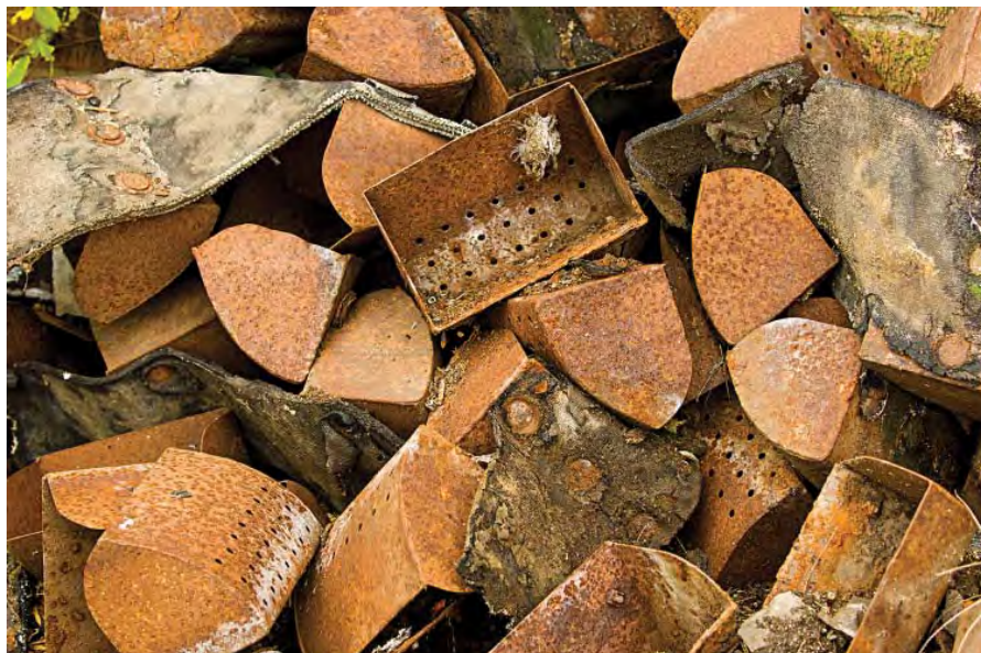
Steel scoops attached to a long conveyor belt called a "bucket elevator" lifted grain high enough to be dumped in a bin. These discarded scoops were at a Fairbury elevator.
