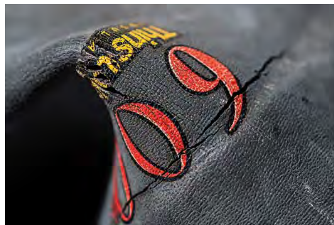
When the boots of waders become cracked, such as this, there is not much that can be done to save them.
