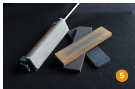
Using progressively finer grit stones, repeat the process for a polished edge.
