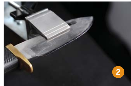
Set the blade parallel to the holding clamps and mark with a felt-tipped pen.
