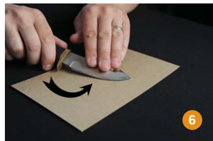
The final step is to strop the blade using leather or cardboard.
