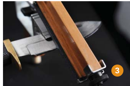
Begin grinding with coarse stone along the entire length of blade to set the angle.
