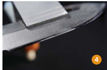
The pen-marked edge will show the areas that need additional grinding.
