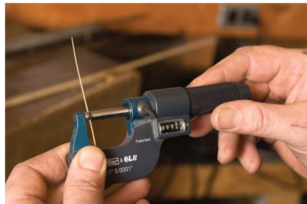
Koch uses a micrometer to check the almost paper-thin ends which will form the rod's tip.
