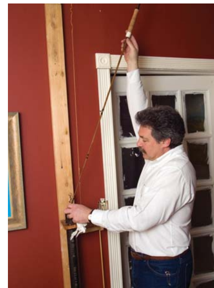
Koch gives an almost-finished rod a coat of varnish to protect it from moisture.
