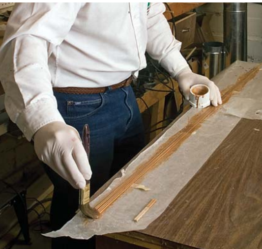
Koch brushes glue onto the inside portion of each bamboo strip.
