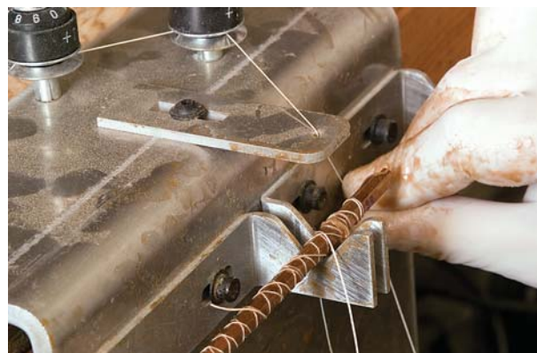
String wound around the six strips of bamboo hold them together in the proper shape while the glue dries.
