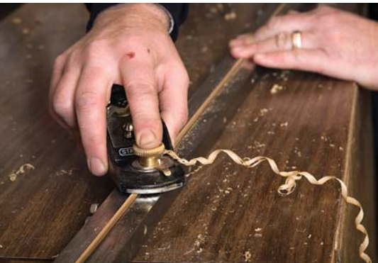
Using a wood plane and planing form, Koch carefully shapes a strip of bamboo.
