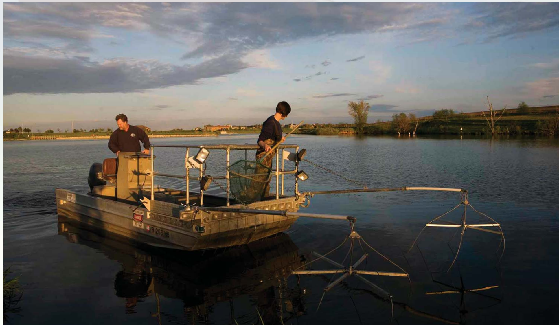
At Prairie View Lake near Bennington, Commission fisheries biologist Larry Pape and conservation technician Lindsey Richters prepare to electrofish just before nightfall. Electrofishing is a survey technique primarily used to analyze black bass populations.
