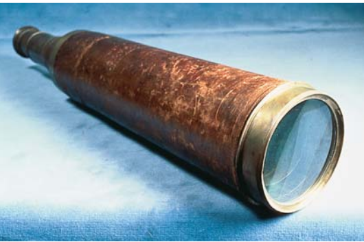
Meriwether Lewis carried this ship's master-type telescope, with five brass and one wood-and-leather collapsible sections, to the Pacific Ocean and back. It was made by William Cary in London in about 1802.
