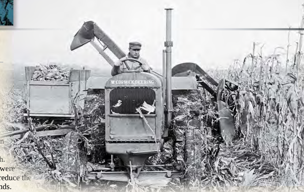
Harvesting with a McCormick-Deering 15-30 tractor (manufactured 1923-29) and a one-row corn picker. Ads claimed the picker "increases your husking capacity six to ten times" over manual husking. History Nebraska RG3358-12s
