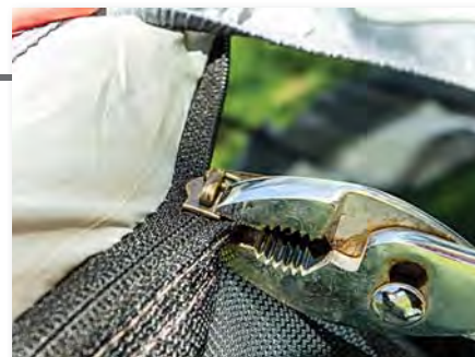
Try to loosen stuck zippers by putting pressure on the pull tab with pliers.
