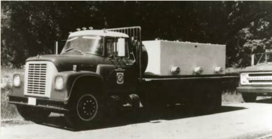
Live trout transport tank on truck from the Rock Creek Hatchery. Undated. NGPC LIBRARY
