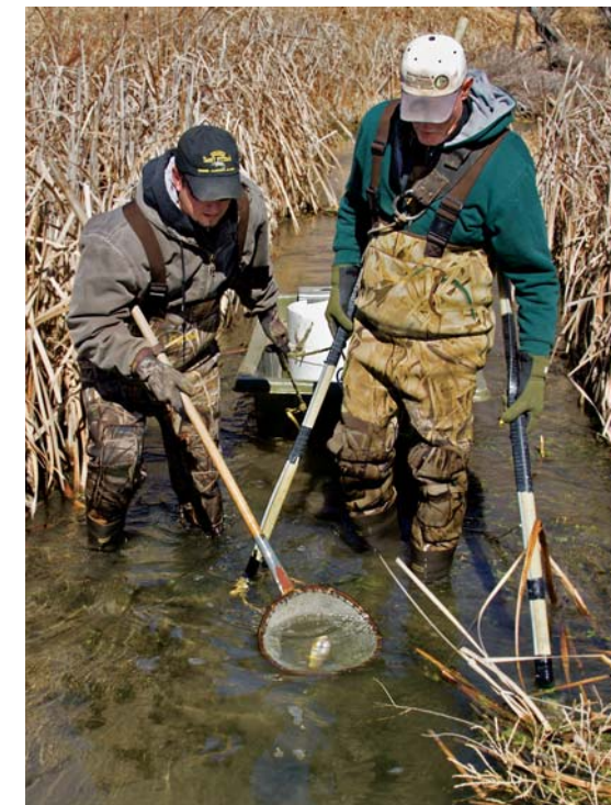
Trout and other fish are momentarily stunned by the electrical current flowing between the hand-held electrodes. Fish captured for the population study are measured, marked, recorded and released back into the stream.
