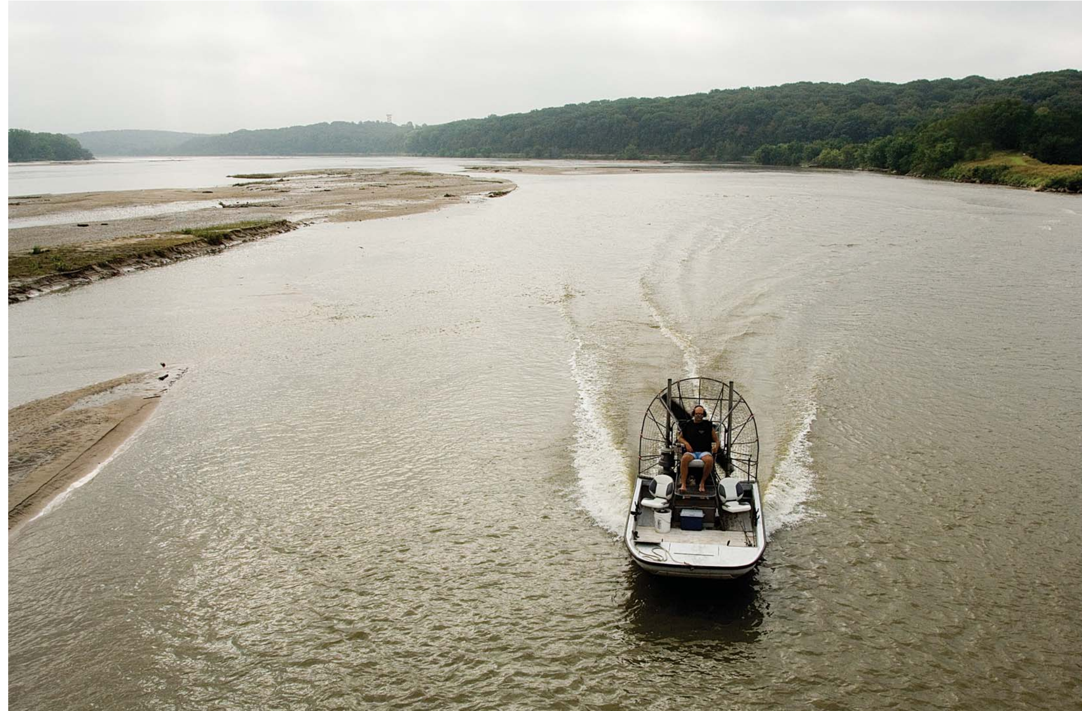
Outfitted with a Lycoming aircraft engine, Ortlieb’s airboat flies down the Platte at a top speed of 55 mph.
