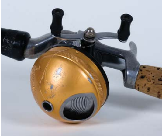
A thumb opening cut into the housing of a promotional Great Lakes reel allowed the angler control of the cast and catch.
