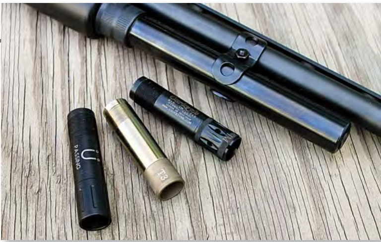
Common upgrades for snow goose guns include high-capacity magazine extensions and long-range choke tubes, such as these from Muller, Rob Robert's, and Carlson's.
