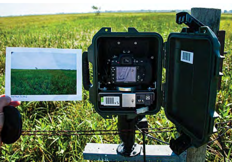
The project's time-lapse cameras are Nikon DSLRs tethered to custom designed technologies in waterproof housings. The first generation (left) images were downloaded by hand and solar power was stored in batteries. Several generations later (right), capacitors are used to store power rather than batteries, and about half the camera systems are delivering images daily to servers by cellular modem.
