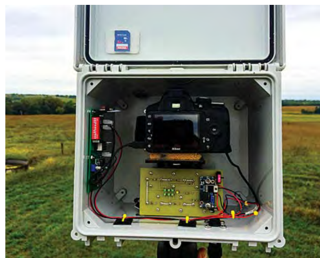
The project's time-lapse cameras are Nikon DSLRs tethered to custom designed technologies in waterproof housings. The first generation (left) images were downloaded by hand and solar power was stored in batteries. Several generations later (right), capacitors are used to store power rather than batteries, and about half the camera systems are delivering images daily to servers by cellular modem.
