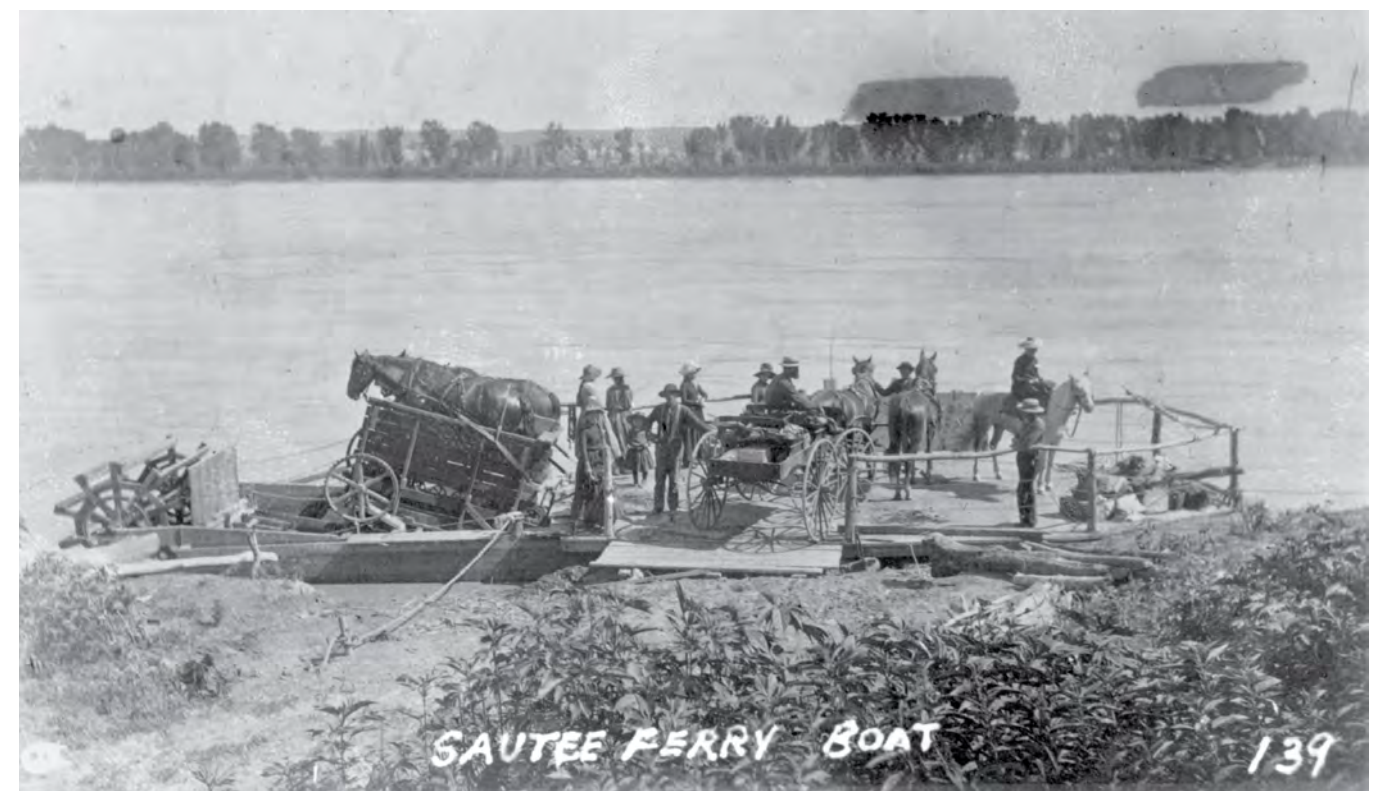
A team boat was propelled by horses on a treadmill. Santee, Knox County. HISTORY NEBRASKA, RG2118-9-8
