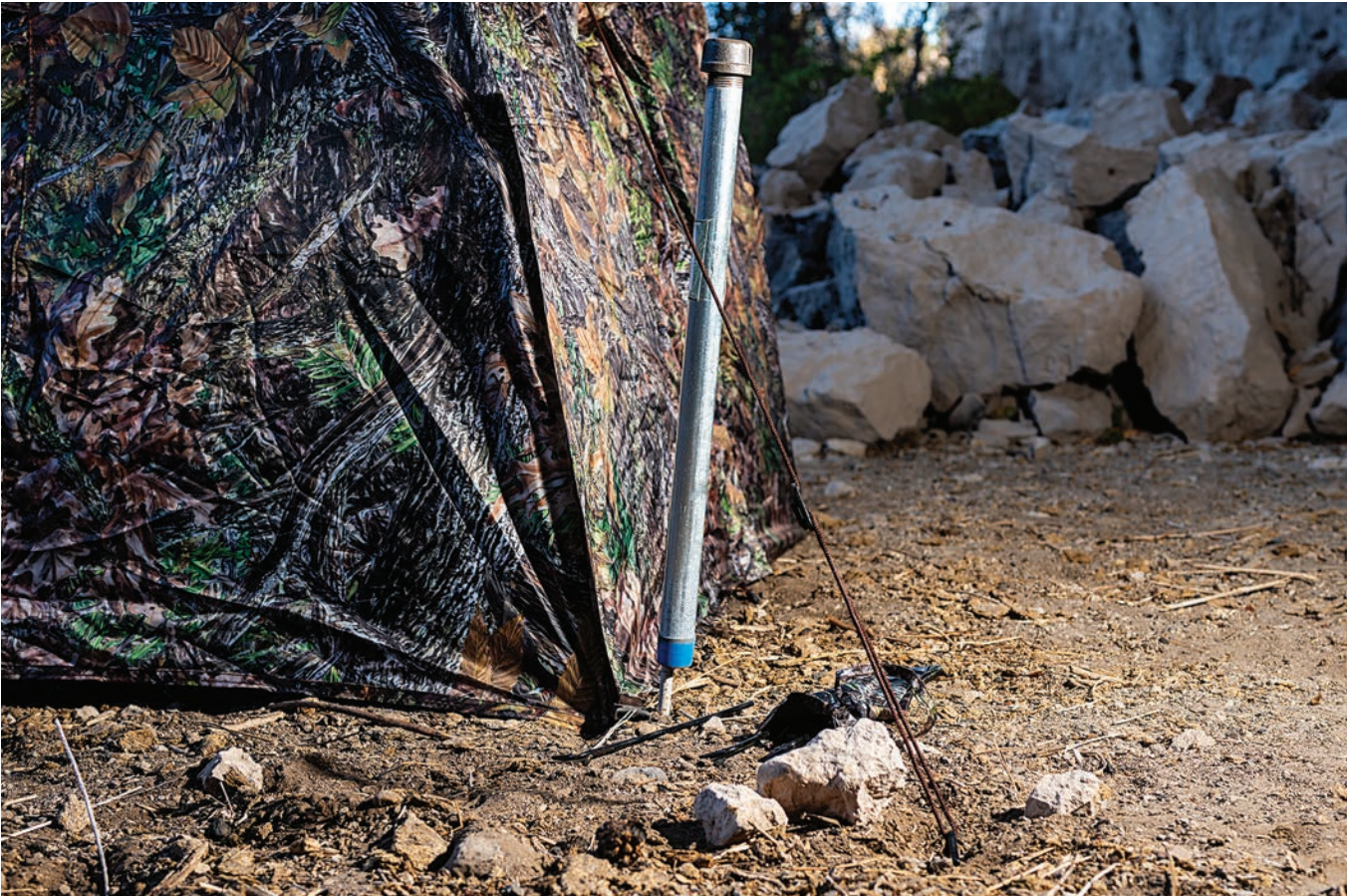
Use a metal pipe and steel rod to create a pilot hole before securing stakes on hard ground. JUSTIN HAAG, NEBRASKALAND
