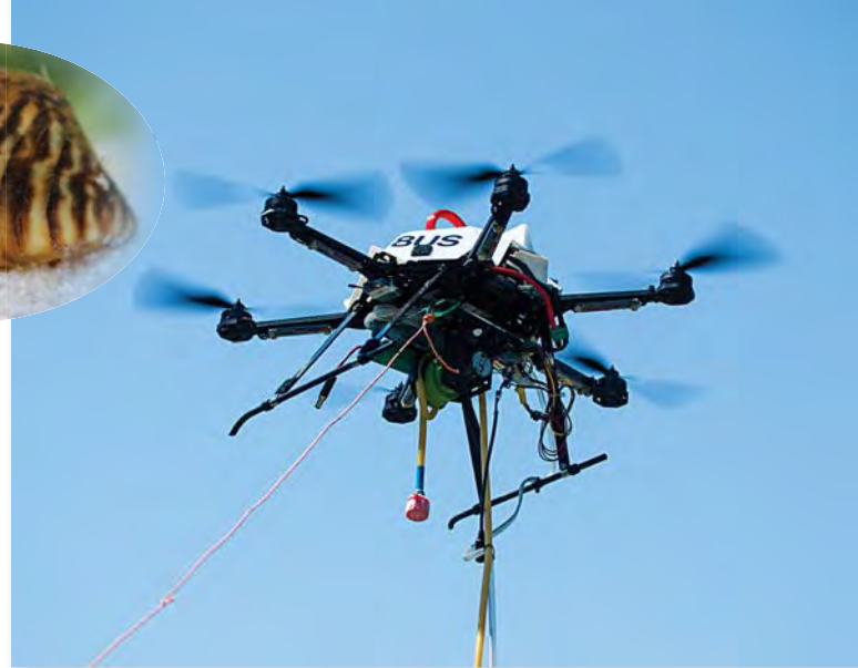
To test for zebra mussels, a drone has been fitted with a pump and filtration system that captures immature mussels.
