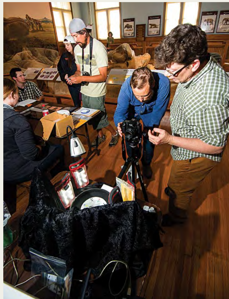
Matthew Douglass and Amy Sobotka photograph a projectile point brought in by a local rancher using a turntable photogrammetry rig. Here the artifact is photographed from multiple angles to allow a 3D reconstruction to be created.
