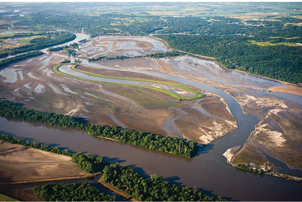
Above: When Missouri River floodwaters receded from Schilling Wildlife Management Area near Plattsmouth last July, the splayed pattern created by the foot of sand deposited by water flowing out of the area's reconstructed chute (bottom right of photo) was plainly visible. High water limited or prevented access to Schilling and other Nebraska Game and Parks Commission areas along the Missouri into fall. Opposite: Heron, raccoon, deer and nightcrawler tracks crisscross the road at Wood Duck WMA near Stanton. Taken six days after the Elkhorn River fell below flood stage, water was still retreating from much of the floodplain.
