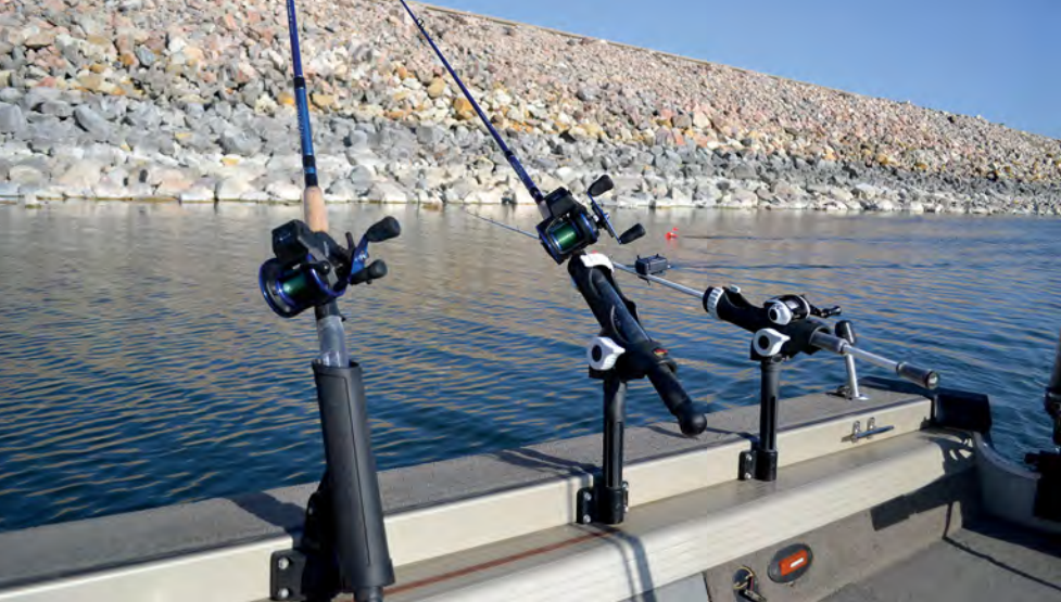
Rod holders maintain and control more than one rod when trolling while also allowing anglers a hands-free option.
