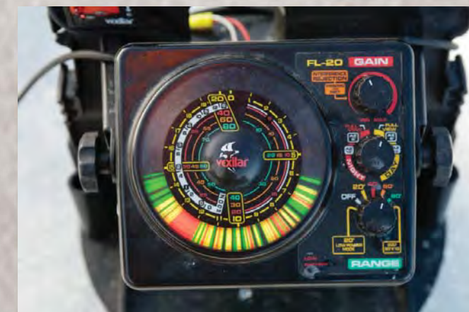
A flasher is a sonar system that provides depth information and reveals the presence of fish or underwater structure.
