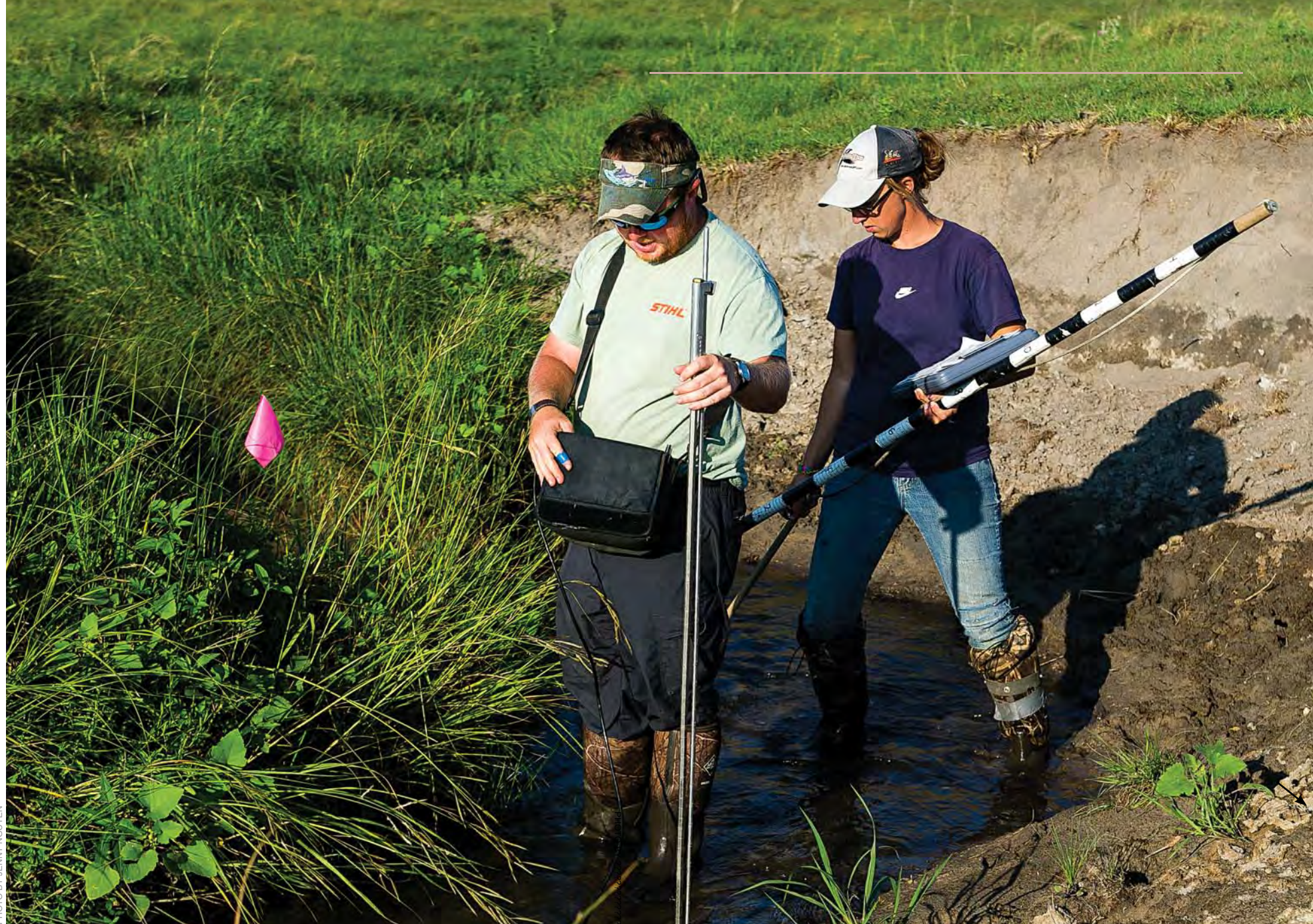
Research technician Miles Arnette from SDSU takes depth and velocity measurements in one of the transects in a Keya Paha Watershed stream. Cassidy Gerdes follows behind to record habitat measurements, including substrate and temperature.
