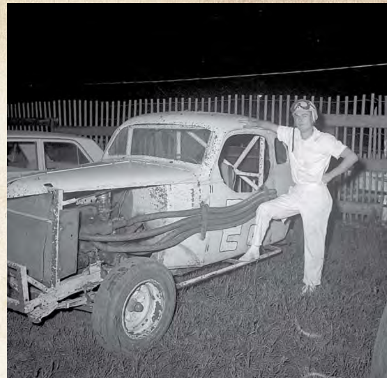
A local racer in Crofton, Nebraska, using flex-hose for exhaust tubing in 1965. RG5705-20-7-2
