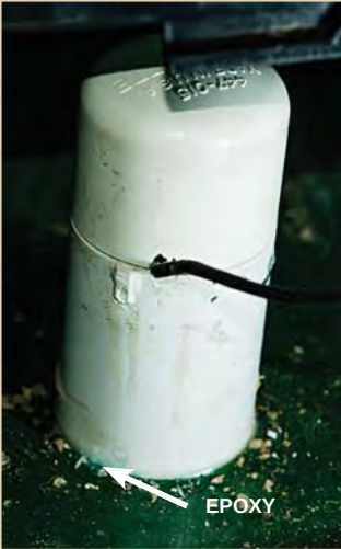
A water-filled transducer housing can be built from PVC pipe and glued to the inside of your kayak's hull.
