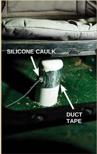
A water-filled transducer housing can be built from PVC pipe and glued to the inside of your kayak's hull.
