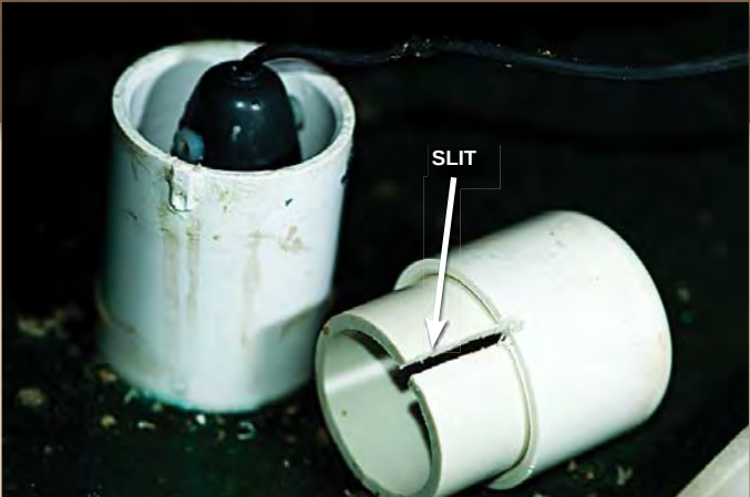
A water-filled transducer housing can be built from PVC pipe and glued to the inside of your kayak's hull.
