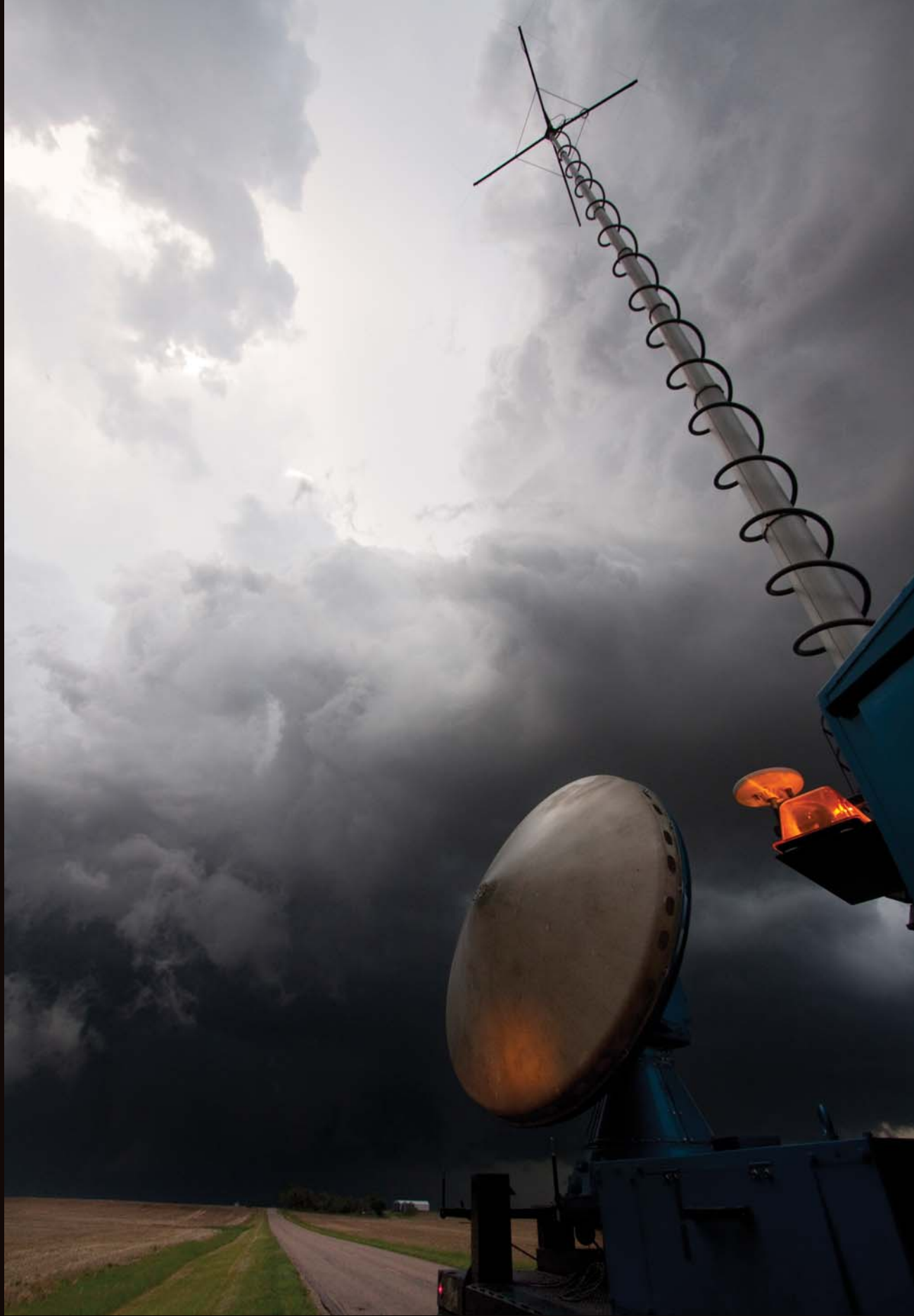
The Center for Severe Weather Research's "Doppler on Wheels" radar truck scans a storm in the Nebraska Panhandle on June 5, 2009, during Project Vortex 2. This radar truck gathers data near tornadoes in an effort to discover why some storms form tornadoes and others don't.
