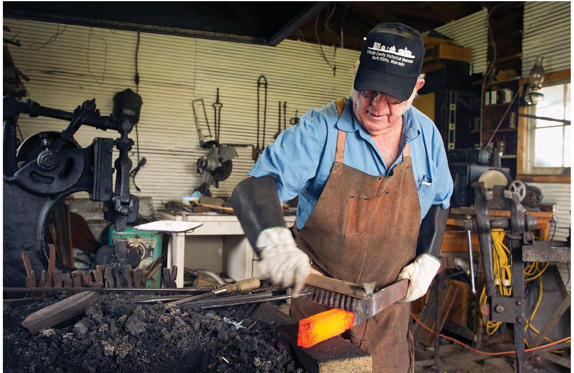
ABOVE: Fanter cleans the hot metal after hammering it with a steel brush to get any debris or slag off the metal, then flux or borax is generously sprinkled on the hot metal to seal any joints off from oxygen. OPPOSITE: Tongs are used to hold the cut billet while Fanter gives the blade its curves with his hammer and anvil.
