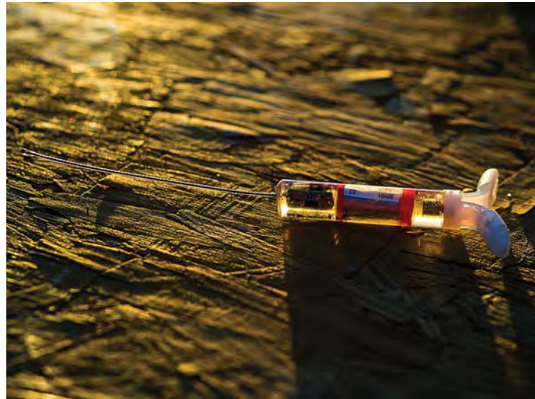
The vaginal implant transmitter is designed to be ejected from a ewe upon the birth of a lamb. A change in its temperature triggers a signal to researchers using telemetry equipment.
