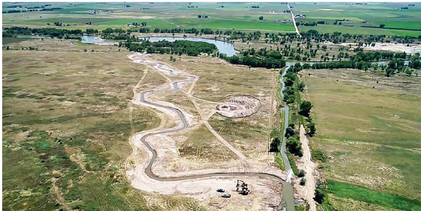
The new trout stream at Dry Spotted Tail Creek meanders to the North Platte River with water diverted from the old straight channel.
