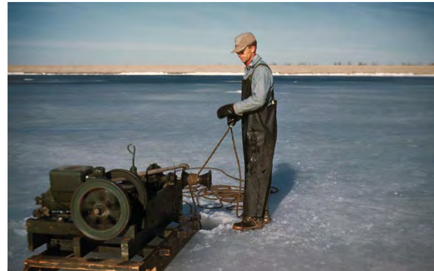
Charlie Koester is pictured using a “pulling jack” gas motor winch built with a Model A Ford transmission and rear end to pull in a net set under the ice in 1959.
