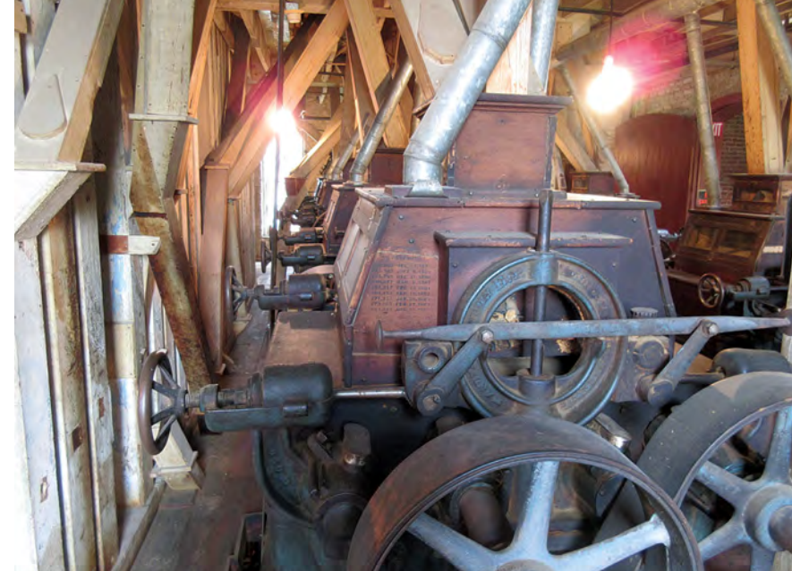
Starting in the mid-1880s, roller mills replaced millstones — also known as burrs — and sped up the milling process. HISTORY NEBRASKA
