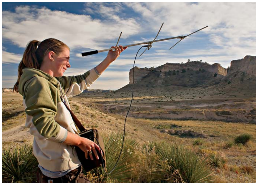
Biologist Holly Kufahl tracks the Hubbard Gap bighorns using a handheld radio receiver and antenna. Each bighorn's radio collar transmits on its own frequency, letting biologists identify and track individual bighorns.
